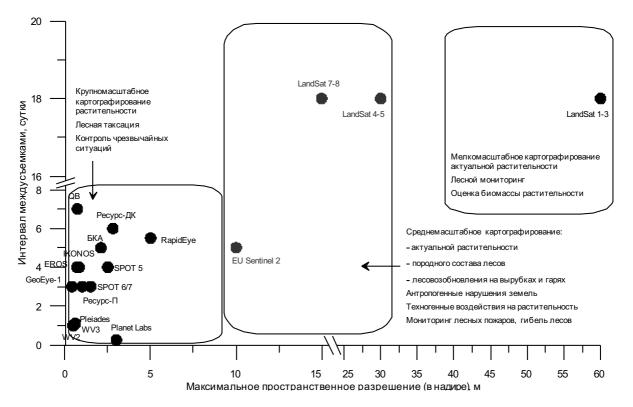
**Fig. 4.** Correlation between spatial and temporal resolution of images and tasks to be solved. Axis Y: Interval between surveys, days; Axis X: Maximal spatial resolution (in nadir), m. First chart dataset: Large-scale
